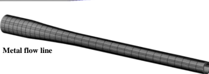
(b) Deformation, effective strain and metal flow line Figure 2.3 Simulation of pilger rolling process
