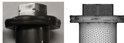
(e) Prediction of wrinkles occurring during bolt head forming
