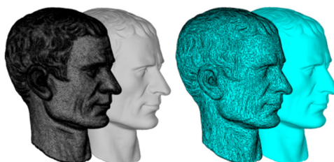
(a) 420,000 tetrahedrons (b) 30,000 tetrahedrons Fig. 1.5 Example of the new coarsening function
