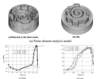
(b) Predicted curve of die tensile stress based on analysis model
